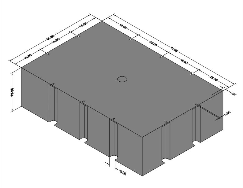
F2150 48" x 72" x 20" 2150 lbs of lift capacity 10 attachment Not UPS shippable
