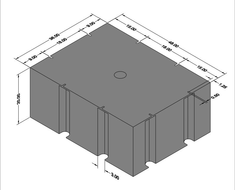
F1100 36" x 48" x 20" 1100 lbs of lift capacity 8 attachment on18" ctrs Not UPS shippable
