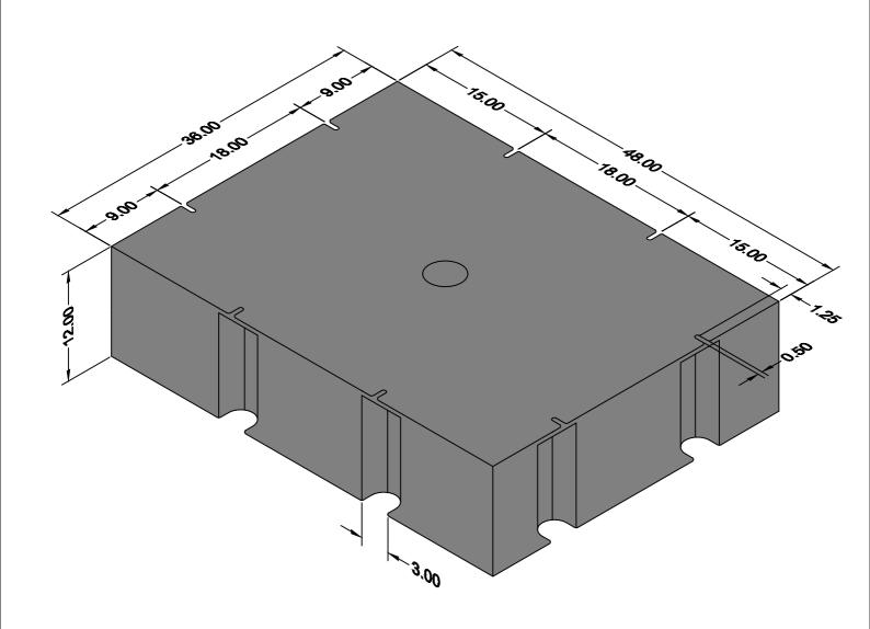
D700 36" x 48" x 12" 700 lbs of lift capacity 8 attachment on 12" and 18" ctrs Not UPS shippable
