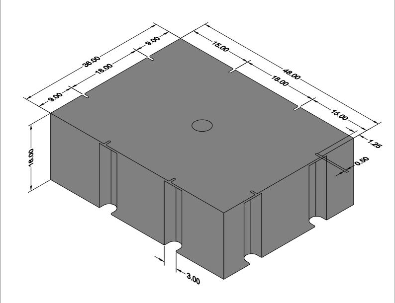
B900 36" x 48" x 16" 900 lbs of lift capacity 8 attachment on18" ctrs Not UPS shippable
