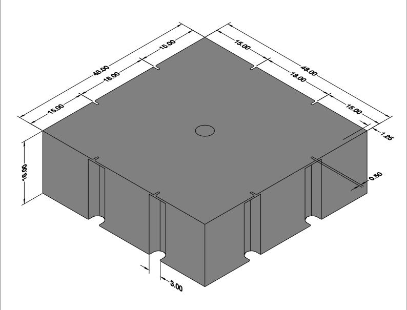
B1200 48" x 48" x 16" 1200 lbs of lift capacity 8 attachment Not UPS shippable
