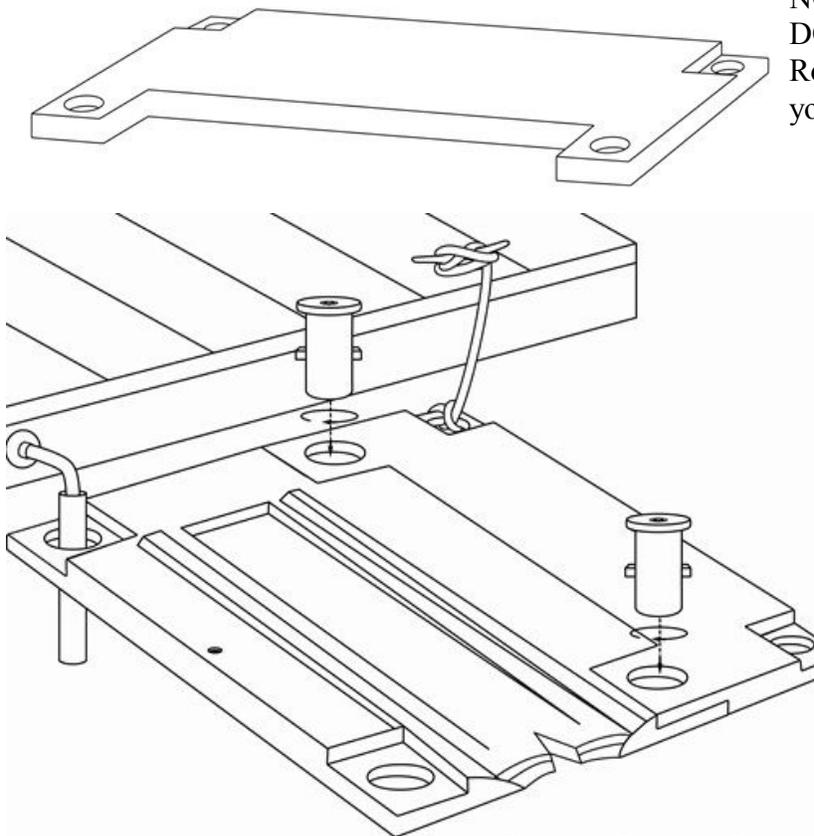
Temporary rope up support bar to watercraft float to prevent bar from falling into water.
