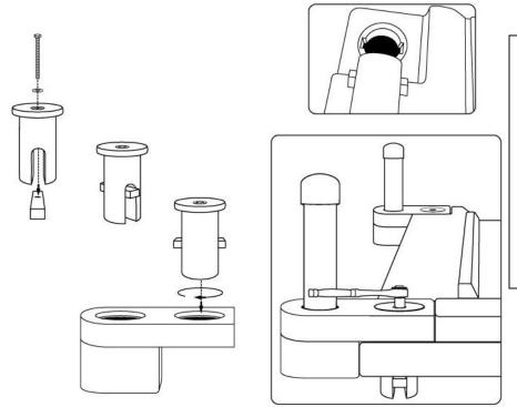
\* Socket Wrench should fit ½" hex Bolt. Run pipe through Pipe Holder kit into lake or sea bottom of at least 2 feet. For rock or clay areas use HDG Pipe and cover with PVC pipe. Some applications may require concrete pour, please consult with your Jetport dealer for any questions
