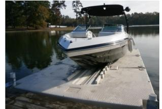
Buoyancy boosters can be added for additional lift in the back if needed. Each set provides 150lbs of additional floatation.
